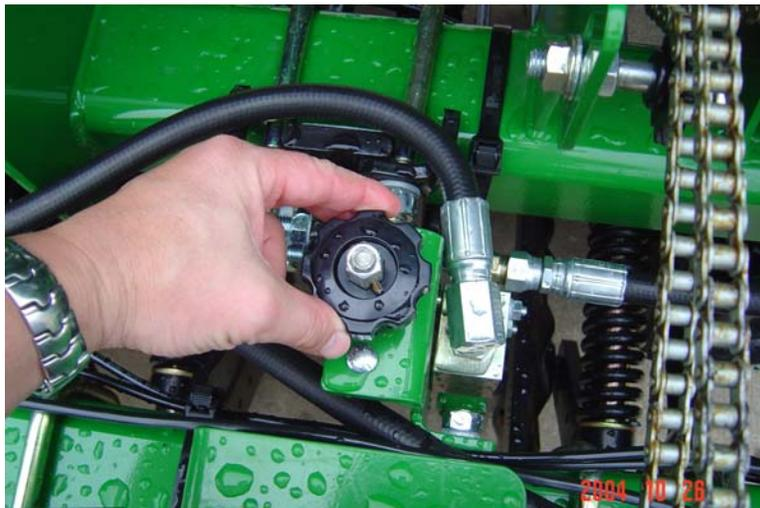
3) 4 Speed Gearbox – The 4 Speed gearbox enables the operator to quickly set up his seed-rates without having to change sprockets.
